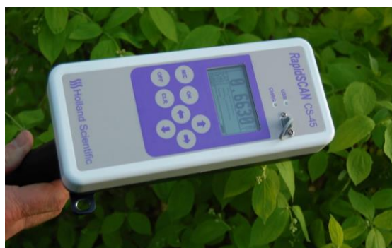
Figure 5: Crop Circle RapidSCAN AC-45 handheld reflectance sensor
