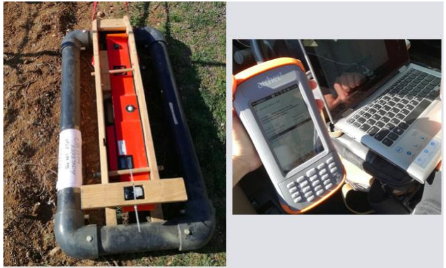
Figure1: EM38-MK2 (left) and Archer Data logger (right)
